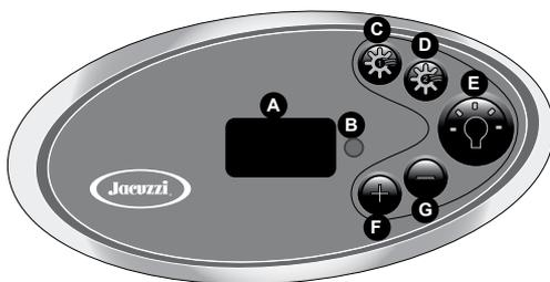
B. **Heat Indicator:** Lit when heater is on.
